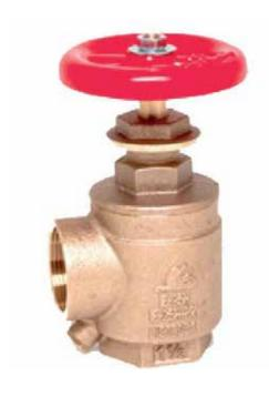
300 lb (2070 KPa) pressure tested approved valve. Heavy Duty 1-1/2" (38 mm) angle hose and hydrola-tor valve.
